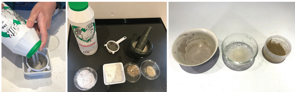
Fig.5 Filtering oyster from shells sand-shell sand, 'white sand' and 'dark sand' Source: Fabricademy class 2020-2021.
