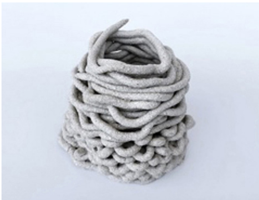
Fig.1 Oyster Shells 3D printed Source: Georgiou, n.d. materiom.org/recipe/609
