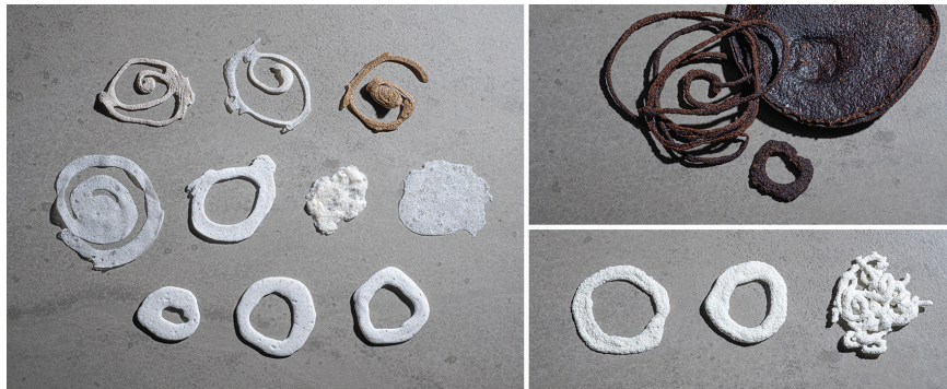
Fig.7 Bio-based composites extruded clockwise: a) Shell sand; b) Coffee grains experiments; white Eggshells Source: Fabricademy class 2020-2021.
