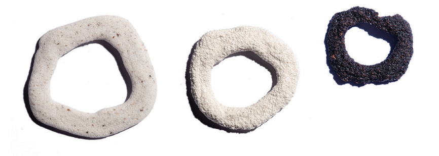
Fig.8 Top – after curing; bottom - two weeks drying - left to right: a) 10 ASS-W8 Shell sand; b) 12 AE - White Eggshells; c) 13 AC - Coffee grains; Source: Fabricademy class 2020-2021
