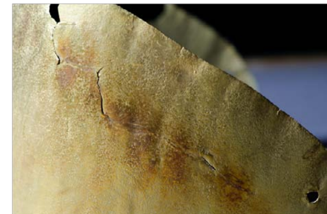
Fig. 2 – Detail of the tarnished surface along a crack of diadem from Évora (Au 133).
