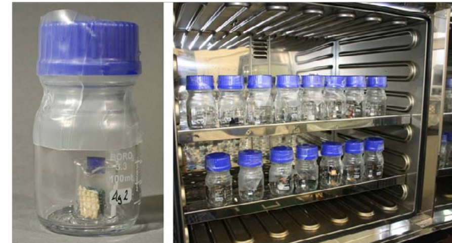
Fig. 3 – Individual set of a glass flask with the copper coupon and a blue fabric sample and the different glass flasks in the oven.
