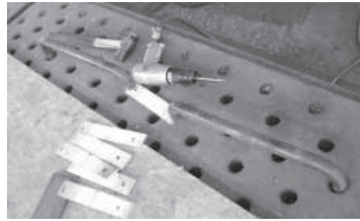
a) Preparation for hammer-peening.
