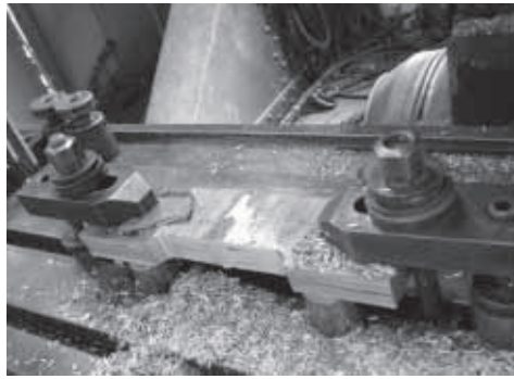
b) Machining of specimens.
