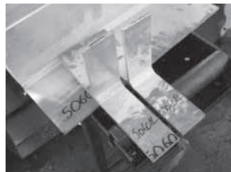
a) “T” joints before Hammer-peening.
