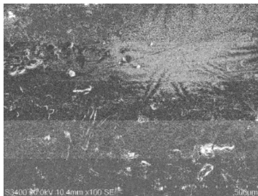
Figure 6a. SEM photograph of mild steel specimen after being corroded in 1 M H 2 SO 4 solution for about 3hrs containing 0.6 mM of BIS.
