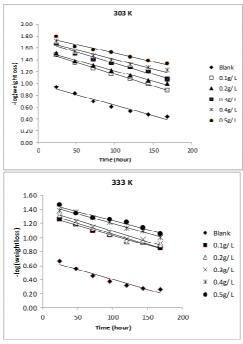
**Figure 6.** Variation of –log(weight loss) with time for the corrosion of Al in 0.1 M HCl containing various concentrations of *FB* gum at 303 and 333 K.
