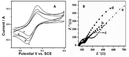
**Figure 3.** (A) CVs of a 5 mM  $Fe(CN)_6^{-3/-4}$  solution obtained for a) bare Gr, b) Gr/PPy, c) Gr/PPy/AgNPs and d) Gr/PPy/AgNPs/PPO. (B) Impedance spectra of a) bare Gr, b) Gr/PPy, c) Gr/PPy/AgNPs and d) Gr/PPy/AgNPs/PPO.
