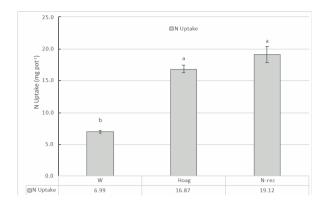
**Figure 2** - N uptake by the triticale in the different treatments. Different letters above de columns indicate statistical differences (*p* <0.05) between the treatments by the Tukey test.
