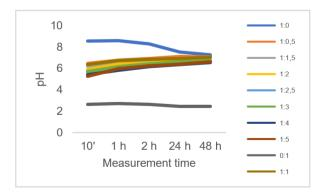
Figure 1 - Evolution of pH for different proportions Technosol and Sulfide tailings (labels on the right represent the ratios).
