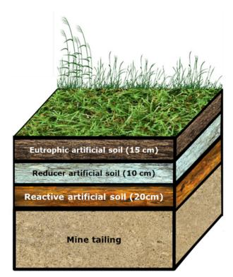
Figure 2 - Design of the artificial soil layers to cover the mine tailing material.
