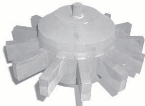
Fig. 21. Demonstration blisc with MC2 single crystal dummy blades integrally bonded to a fine grain U720 hub.
