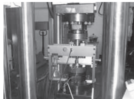
Fig. 4. Fretting fatigue experimental test setup [19]
