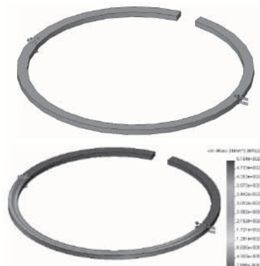
Fig. 2. a) Piston ring (applied load and restraints); b) Stress distribution on a piston ring
