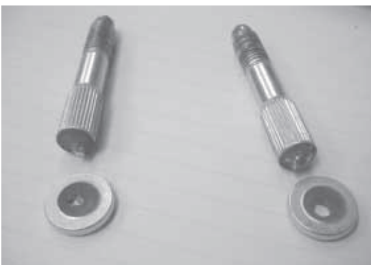
Fig. 1. General view of two fractured bolts
