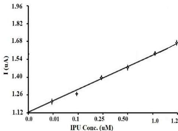
**Figure 6.** SWV calibration plot with successive increases in IPU concentrations.
