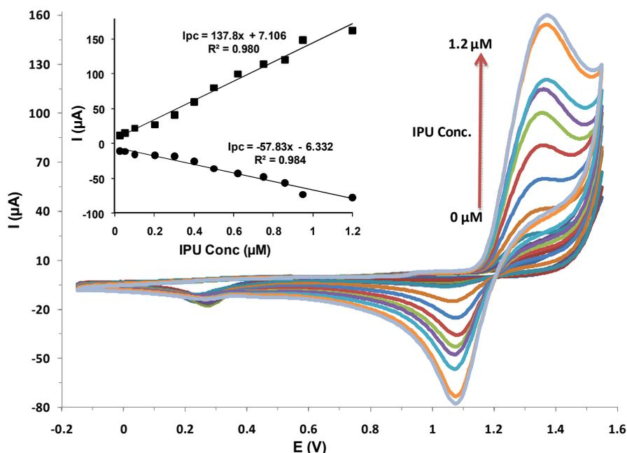
**Figure 4.** IPU CV on PNC/GCE in 1 M HClO<sub>4</sub> (pH 2), with successive increases in concentration from 0.01, 0.025, 0.05, 0.075, 0.10, 0.20, 0.30, 0.40, 0.60, 0.80, 1.0 to 1.20  $\mu\text{M}$ , respectively.
