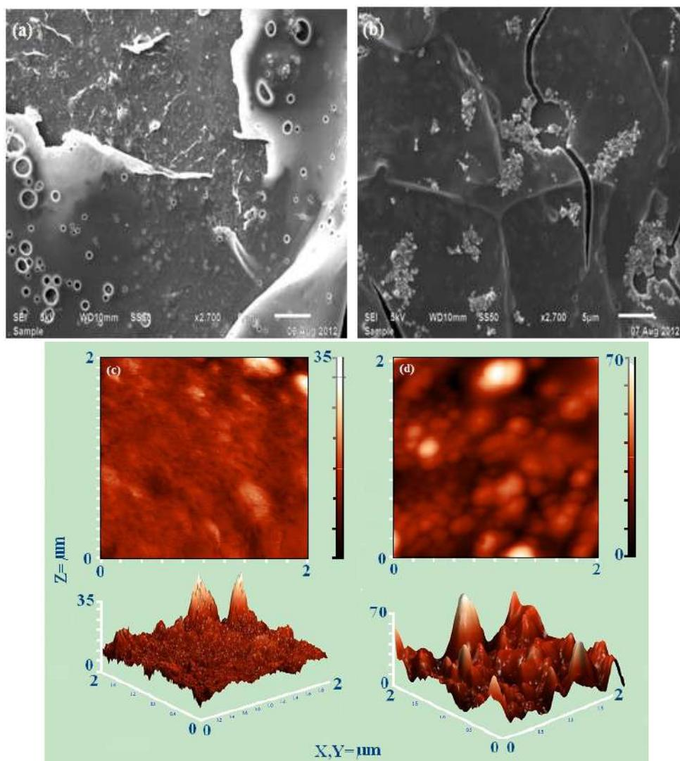
**Figure 1.** SEM of (a) PMMA; and (b) PNC. AFM of (c) PMMA; and (d) PNC.
