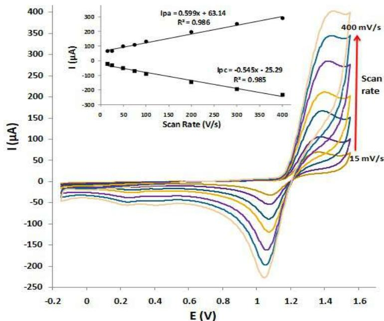
**Figure 3.** IPU CVs of on PNC/GCE, at a scan rate varying from 15 mV to 400 mV, in 1 M HClO<sub>4</sub> (pH 2).
