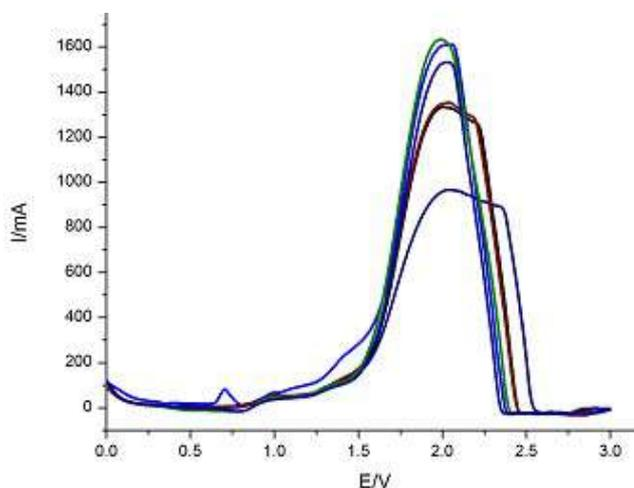
**Figure 5.** IPU SWV on PNC/GCE with concentrations ranging from 0.025 to 1.2  $\mu\text{M}$ , in 1 M  $\text{HClO}_4$ , at pH 2.
