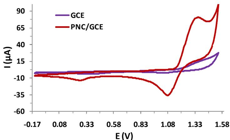
**Figure 2.** IPU CV on GCE and PNC/GCE in 1 M HClO<sub>4</sub>.
