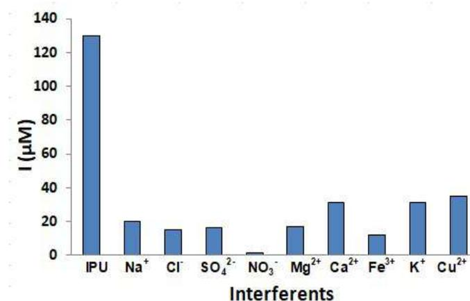
**Figure 7.** Comparative amperometric response of common interfering ions on IPU estimation at PNC/GCE.
