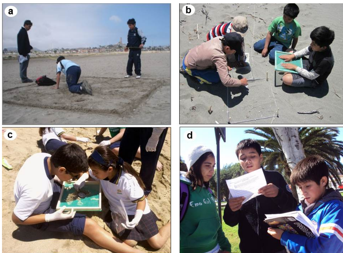
Figure 2 - (A) Sampling for macroplastics. (B) Sieving of sand for microplastics. (C) Sorting of microplastics from material retained in the sieve. (D) Recording the answers of interviewees; one kid asked the questions, while the other wrote down the answers.
